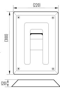
The loop is fabricated from 20mm solid galvanised steel plate and is therefore extremely strong and durable. The Motorcycle Locking Loop - Bolt Down is finished in galvanised mild steel making it ideal for use outside where it will retain it's looks for years.
