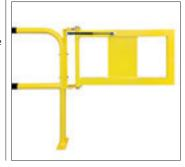
These additions to our popular range of Hoop Guards are manufactured in 40mmØ steel with a 1.5mm wall thickness. Ideal for areas which require less heavy protection as provided by our standard range of Hoop Guards. Intended for indoor use only they are finished in an eye-catching powder coated yellow with black bands. Quickly and easily installed using 8 fixing bolts per guard.
