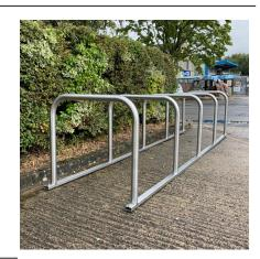
The Sheffield Cycle Toastrack is a floor fixed cycle rack based upon the Sheffield Cycle Stand. The Sheffield Cycle Toastrack consists of Sheffield Cycle Stands welded at 800mm centres to floor fixed box section rails. The benefits of a Cycle Toastrack over individual stands are reduced installation costs and pre-determined gaps between stands, each stand is suitable for parking two bicycles. The Sheffield Toastrack is ideal where cycle parking in large numbers is required.
