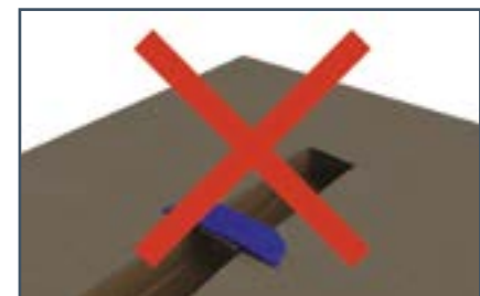
The End Piece is not load bearing and must be entirely on solid ground.
