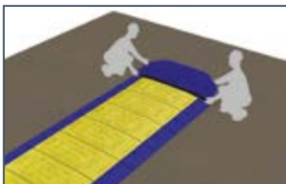
If required - Connect the End Piece. It is light enough to be installed without the EasiLift handles
