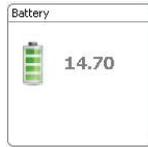
Battery level indicator: In case of low battery, the color of the icon changes. A fully charged battery is between 12.8V and 13.1V
