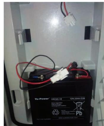
**Power autonomy** – One sole battery will generally provide sufficient power for 3 to 8 days dependent on traffic flow. The radar will indicate low-battery by showing a tri-colored square
