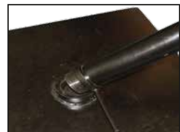
Securing Tube is screwed into the Base Plate
