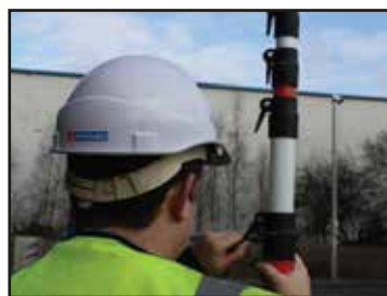
Multiple Clamping System with sturdy reinforced fibreglass sections with metal hooking system for bunting and/or crossbar
