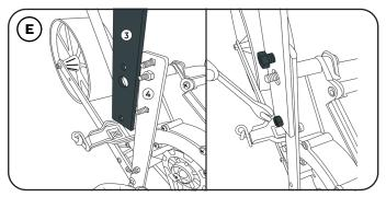
Align the holes of item 3 (Handle Section) with the bolts protruding from item 4 (main body frame). Place item 3 (handle section) onto item 4 (main body frame) and tighten the highlighted nuts.
