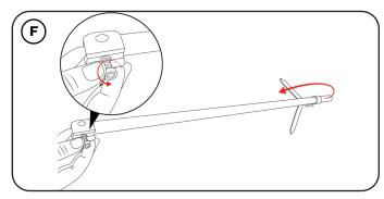
Take item 5 (row marker arm) and remove the nut located at the bottom end.
