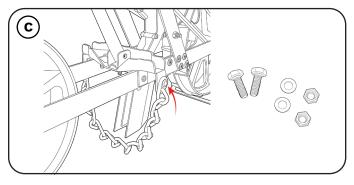
Using provided screws, washers and nuts, attach chain on both sides to the row marker mounting bracket as shown.
