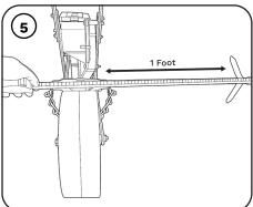
Adjust the row marker to the correct distance as shown.
