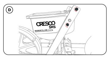
Remove the highlighted nuts from item 4 (main body frame). Remove the same nuts on the reverse side.
