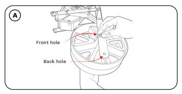
Remove the long bolt located through the middle of item 2 (rear wheel). Re attach the wheel to the back hole on item 4 (main body frame).
