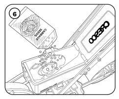
Empty the seeds into the hopper but make sure you do not exceed the maximum fill line. Overfilling can result in over application which will damage your yield.
