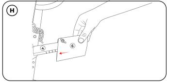
Take item 6 (Depth setting blade) and loosen the wing nut slightly. Slide item 6 (Depth setting blade) onto the depth marker protruding from the bottom of item 4 (main body frame).
