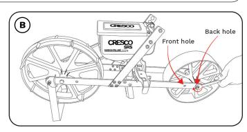
Align the centre hole of item 2 (Rear wheel) to the back hole of item 4 (main body frame). Tighten nut to secure item 2 (Rear wheel).
