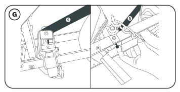
Place the bolt protruding from item 5 (row marker) into the hole shown on item 4 (main body frame). Secure item 5 (row marker) with the nut you removed instep E.
