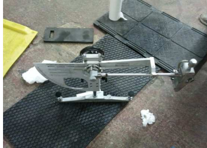
Image 1. Pendulum tester in-situ
