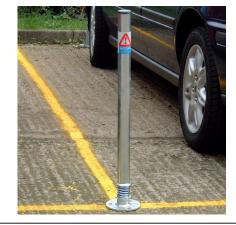
Designed for use delineating the edge of car parking spaces, the Sprung Boundary Post has a spring incorporated into the base which allows it to absorb low speed impacts and return to it's original upright position.
