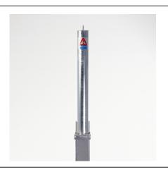
The RetractaPost is a simple, cost effective, yet highly effective way to prevent unwanted vehicle access. The RetractaPost is raised and lowered vertically. When lowered the post is fully below ground and covered using the integral lid. The post is padlockable (padlock not supplied) in the raised position by first rotating the post 45° and then attaching the padlock between the post to the lid. The RetractaPost 745 is 745mm above ground in the raised position.
