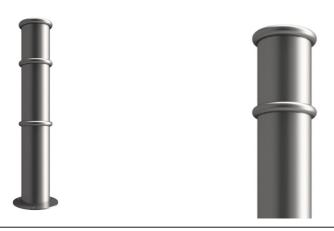
The GFC6000 Ornamental Mild Steel Bollard from AUTOPA is suitable for a wide range of locations and purposes. Constructed using mild steel, then galvanised to ensure its longevity. Cap and rings are welded onto the steel tube to complete the design.
