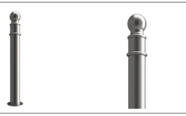
The GFC5000 Ornamental Mild Steel Bollard from AUTOPA is suitable for a wide range of locations and purposes. Constructed using mild steel, then galvanised to ensure its longevity. Cap and ring are welded onto the steel tube to complete the design.
