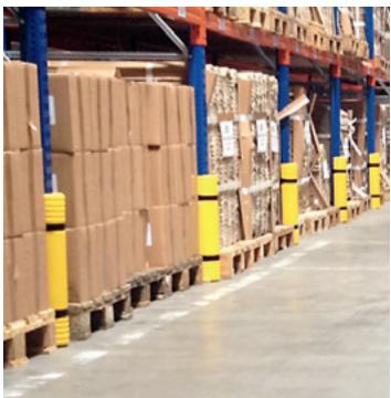
Impact Protection for pallet racking uprights manufactured from high quality polyethylene. Easily and quickly secured by two Velcro straps – no drilling into the floor required.
