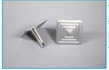
The stainless steel crossing studs are also 100mm square and have a serrated finish to improve skid resistance in adverse weather conditions, and have a fishtail shank.
