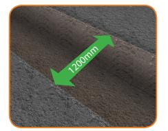
Ensure max trench width less than 1200mm. Assess trench stability prior to install.
