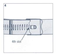
Locate the tongue of the buckle in the 4th slot of the band. Screw the band through using a hand or power tool.
