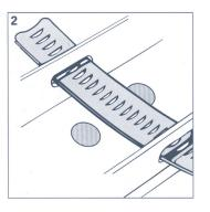
Thread the band through the slots in the sign and around post.
