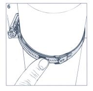
Push any remaining excess band through the buckle for a safe, tidy job. Tamtorque can be released and repositioned if required.
