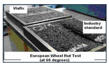
Image shows comparative performance of water activated Viafix versus a market leading solvent-fluxed cold lay material. The exceptional performance characteristics of Viafix make it the best option for reinstatements in all circumstances.
