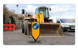
We recently tested the resilience and durability of our Evo-N traffic bollard against a 7 tonne JCB. On the day we hit the bollard time and time again. The EVO-N took every bit of punishment from the 7t heavy plant in this extreme test, and then stood straight back up again. If we'd continued the JCB would probably have run out of diesel before the Evo-N would have stayed down.
