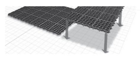
Ecogrid is both swift and easy to lay without the need for specialised machinary. The system is delivered in palletised form in layers of 12 grids or 1.33 sqm pre-locked together. These layers are taken off the pallet by one person, offered to the ground, the next layer simply snaps firmly in to place with foot pressure.
